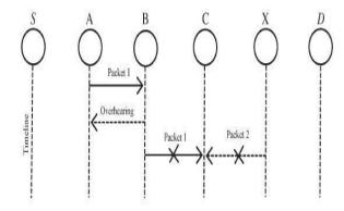
Figure 2: Receiver Collision
